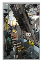
At the same time of the lines formation, the draw arm pick up the carton and is folded during the drop down on principal carton transport chain belt.
