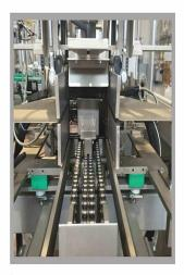
After the filled carton move forward to the second station, the squaring group will complitaly close lateral strip, glued (by format) during the transport chain belt movement.
