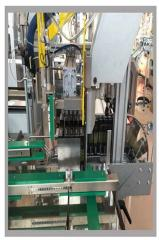
After reaching the settings number of products, the line goes into the moulding former area, through the lateral pusher, created the requested number (by format).
