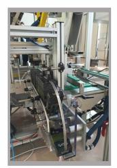
The product (cases) exiting from the start machine on lines enter in the slide valves alimentation belt, rounded of 90° and aligned.
