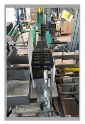
Later, the carton is sideways filled by the lateral pusher, with the products prepared at the start. During the shift of the pusher and the products insertion, the top longitudinal strip of the carton get alued.
